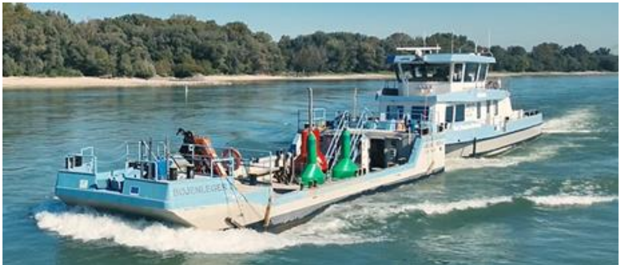
Figure 7-2: The Bad Deutsch-Altenburg pushing a barge carrying waterway marking equipment.
