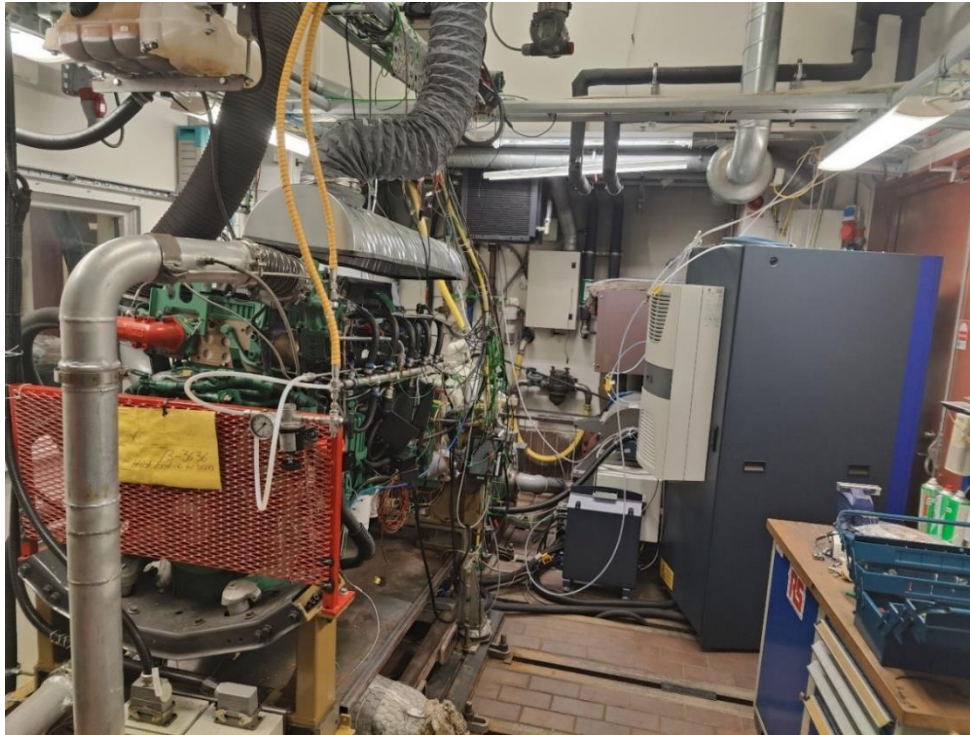
5 | Arrangement of the engine in the test dyno
