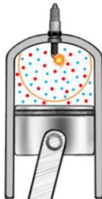
Figure 26 Hydrogen Mono-fuel engine with spark ignition. Here, nearly zero-emission is possible. A high lambda value is required for low NO x emissions and high efficiency. Mono-fuel engines tend to be larger than dual-fuel engines due to reduced power output [27]. Red resembles oxygen, blue hydrogen and orange the emerging NO x .
